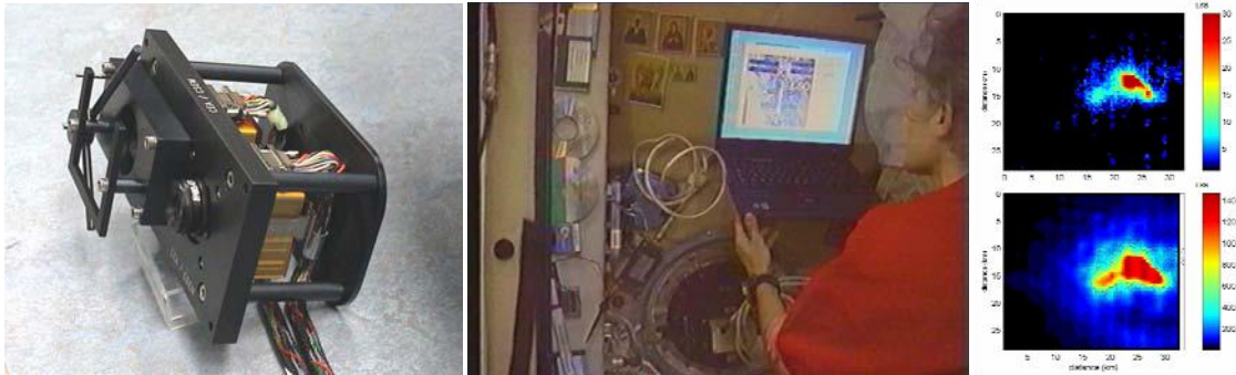
Fig. 6. Left: Micro-cameras, mechanics and filter holding system for LSO. Center: Instrument operated by the astronaut. Right: Images of sprites obtained with LSO (credits CEA).
