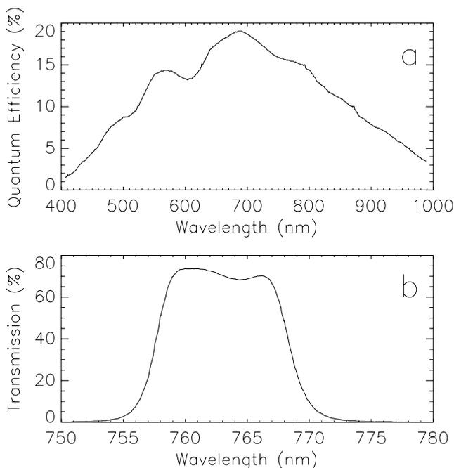
**Figure 2.** Spectral response of the LSO microcameras and of the filter.
